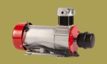
200 psi max pressure Weight 20 lbs / 9Kg Size H172xW106xL276 6 CFM @ 0psi / 2.6 CFM @ 100psi 82 amps draw @ 100 psi
