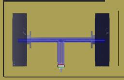
Applicable to all vehicle without CTIS hub Simple adaptive air path hub to wheels Rotating seal inside the axle No external exposure No axle oil contamination
